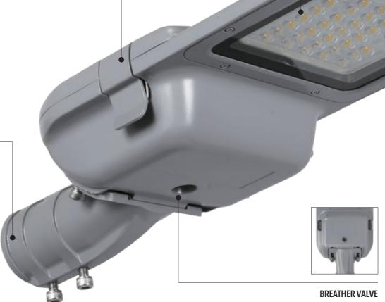
The electrical compartment is equipped with an advanced breather valve for improved waterproof and heat dissipation performance.
